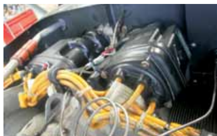
Magneto and wiring.
