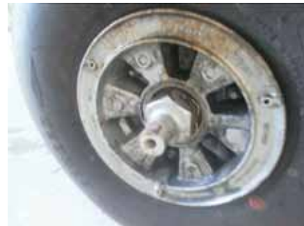
Main wheel and cotter pin location.
