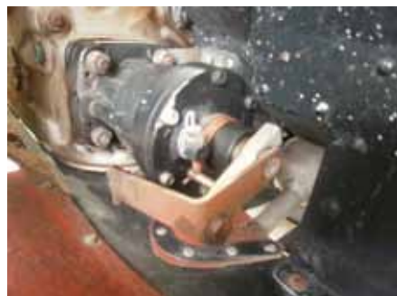
Propeller governor and linkage.
