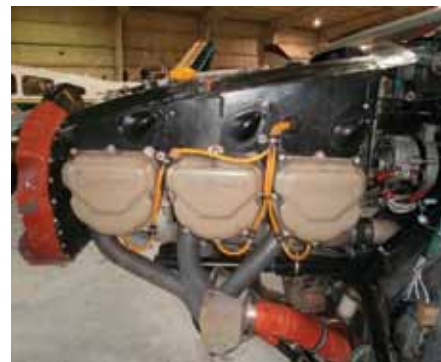
Preparing the engine for a compression check and spark plug removal.
